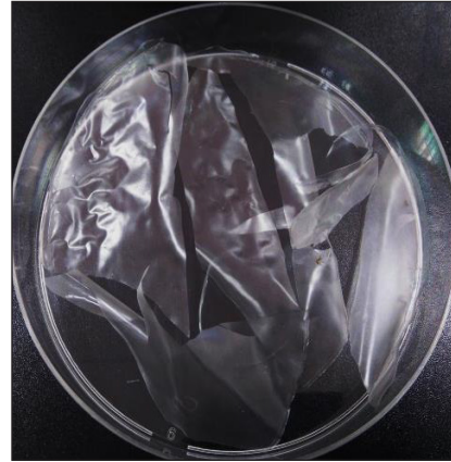
Figure 1. Neat tapioca starch film without the addition of glycerol
